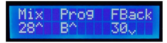
The  $^{\circ}$  and  $^{\vee}$  characters that you may see beside each number indicates if the parameter knob value is currently lower ( $^{\circ}$ ) or higher ( $^{\vee}$ ) than the value currently stored with the patch. Think of the arrow as an indicator telling you to increase ( $^{\circ}$ ) or decrease ( $^{\vee}$ ) the control setting to match. You can ignore these
