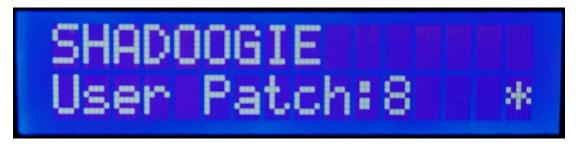
The P1 knob will now be 'live' allowing you to tweak the dry/echo mix. When in this mode the setting of the P1 knob temporarily overrides the value stored in the patch. **NB: YOU CANNOT CHANGE PATCHES WHILE IN THIS MODE.**
