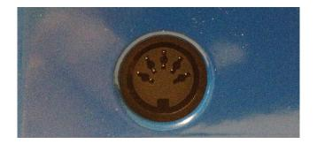
By connecting the MIDI Out from your computer, MIDI keyboard or foot controller to the **MIDI IN** on the Blue Nebula using a standard MIDI cable, you will be able to send *program change* (PC) messages to select different user patches.
