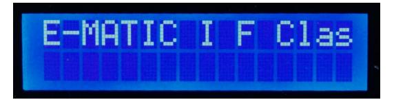
You can change this if you wish by this using the **UP** and **DOWN** buttons to select any of the 16 effects available in the Blue Nebula. With the required effect displayed hit the **OK** button to select it and the top line of the display will now show the names of the effect's parameters with the current values of the three parameter adjust knobs P1, P2 and P3 on the bottom line:
